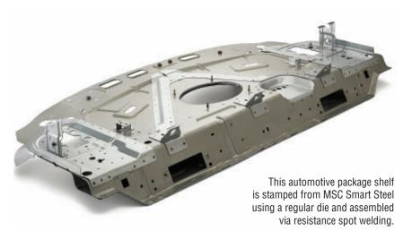
The OEM dictates the design and performance requirements of each component in the vehicle. As a result, MSC engineers work closely with OEM design teams for material selection, joint design, fatigue and strength criteria, as well as weight targets, Murphy said.
